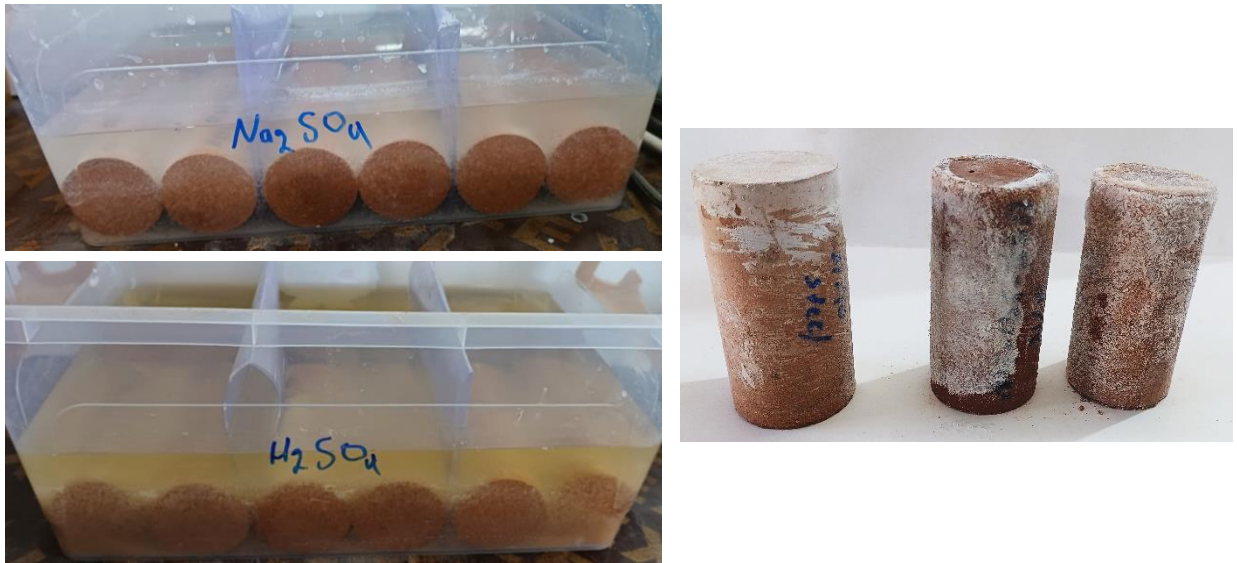
Figure 6 compressive strength of geopolymer samples immersed in H 2 SO 4 and Na 2 SO 4 solutions.
