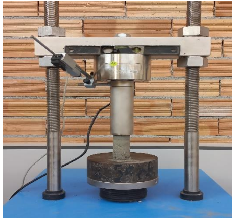
Figure 3: Unconfined compressive strength samples.
