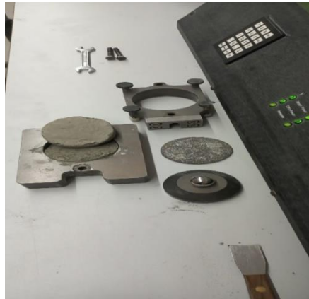
Figure 5: Direct shear strength samples.
